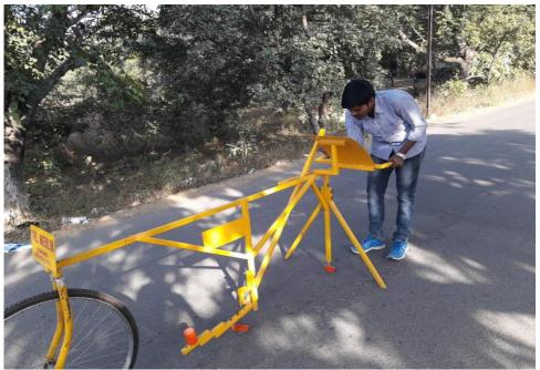
Machine Evaluating Roughness using Low-cost Instrumentation (MERLIN)
