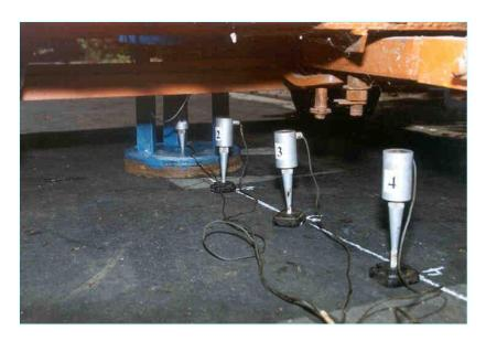
Falling Weight Deflectometer (FWD) - A Low cost model
