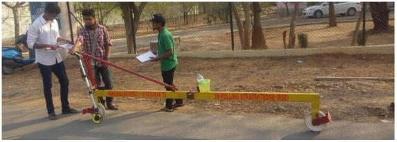
Measurement of Unevenness of Roads in Osmania University by Using **ELECTRONIC 3-M ROLLING STRAIGHT EDGE (ERSE)**
